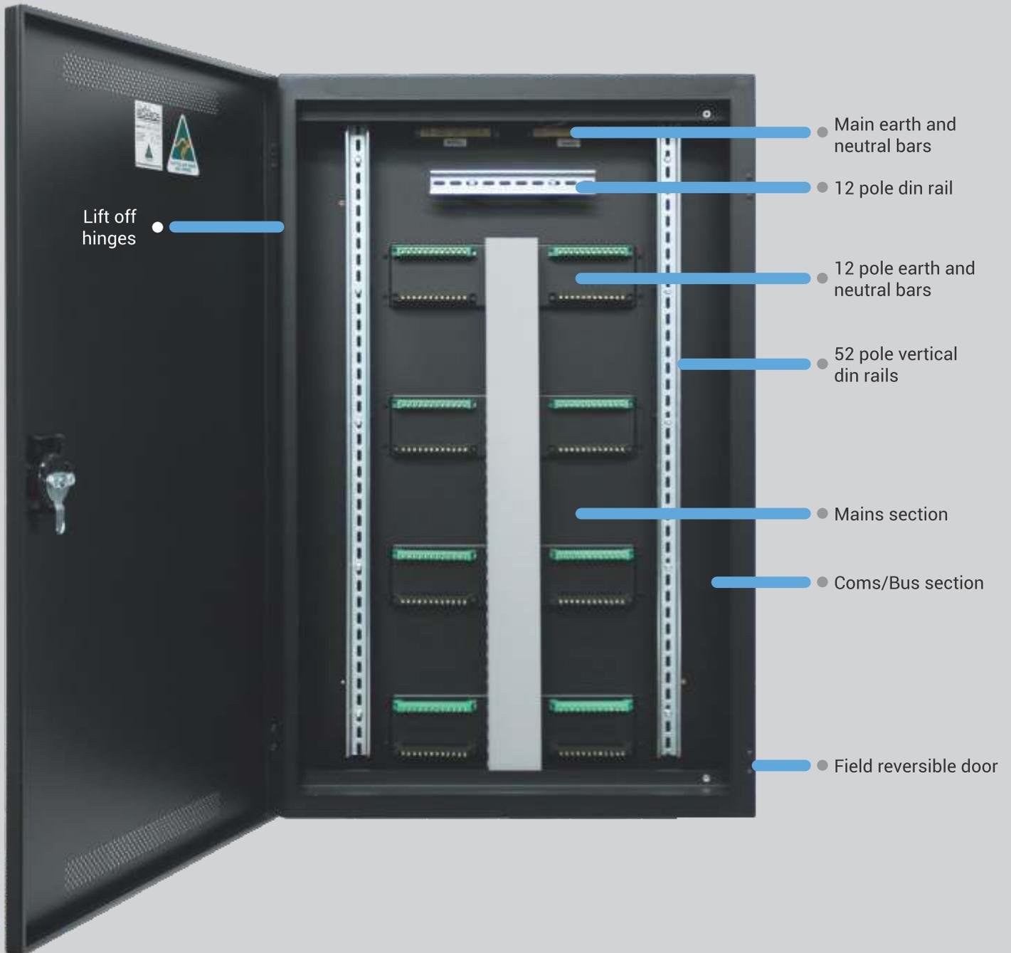
This new enclosure has been developed to use with Control 4 Hardware. The design allows for the hardware to be installed vertically. The Com/Bus wiring and connections run around the outside to solve the issues of segregation from the mains wiring at the top and down the centre.
