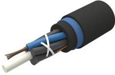
Fiber Optic Cable, Singlemode Outdoor, Triple Jacket, Anti Termite, All-Dielectric Gel Filled, Mini Stranded Loose Tube
